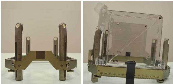
FIG. 1. Leksell stereotactic coordinate Frame G: (left) frame assembled with the curved front piece in the upwards position, angled anterior insulated posts and medium straight insulated posts posteriorly; (right) lateral view of the Leksell Frame G with the MRI fiducial indicator box attached.
